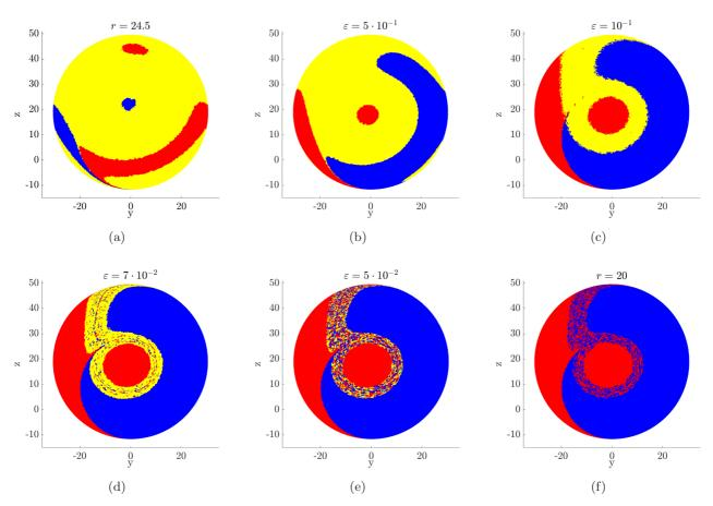
Fig. 9. Rate-induced tipping phenomenon. The scenario-dependent basins of attraction for different values of  $\varepsilon$  showing that for high parameter change rates a significant number of trajectories tip to the chaotic attractor. We also show the basins of attraction of the frozen-in system for r=20 and r=24.5 for comparison. In all cases we have fixed  $t_1=0, r_0=20$  and  $r_f=24.5$ .
