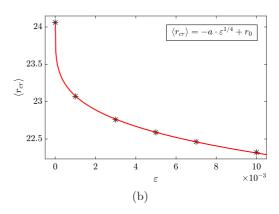
Fig. 7. Critical value of the parameter r and scaling law for the heteroclinic dynamic bifurcation. (a) The normal distribution of  $r_{cr}$  for an ensemble of trajectories with a specific rate of change of  $\varepsilon = 10^{-3}$ . (b) The mean value of  $r_{cr}$  for different values of  $\varepsilon$ . The stars correspond to numerically calculated values of  $\langle r_{cr} \rangle$ , the power law fit is also shown in red.
