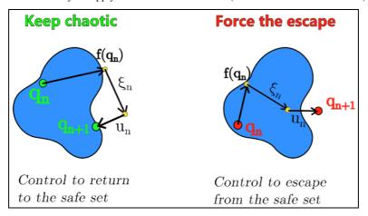
Notes: In this figure, we represent a scheme of the safe set and how the control is applied. We assume that some disturbance  $\xi_n$  is affecting the dynamics, so that  $q_{n+1} = f(q_n) + \xi_n + u_n$ . In the figure on the left, the goal of the control  $u_n$  is to go back to the safe set to keep the chaotic transient behaviour. In the figure on the right, the control is applied to push aside the orbit from the safe set and therefore produce the escape.
