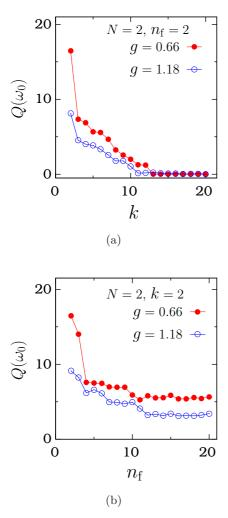
Fig. 12. Plots of (a)  $Q(\omega_0)$  versus k for  $n_f = 2$  and (b)  $Q(\omega_0)$  versus  $n_f$  for k = 2 in S(t) given by Eq. (1) and for g = 0.66 and 1.18 in the first and second resonance intervals. At these two values of g the response amplitude,  $Q(\omega_0)$  becomes maximum for N = 2,  $n_f = 2$  and k = 2.
