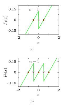
Fig. 1. Sawtooth functions  $F_1(x)$  and  $F_2(x)$  given by Eqs. (2d) and (2e) respectively with n = 1,  $\xi = 0.25$ and A = 0.5. The solid circles and the symbol "×" mark the locations of the equilibrium points and the breakpoints, respectively.
