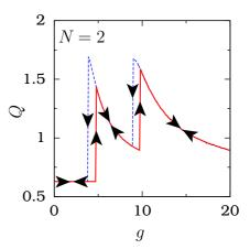
Fig. 3. Resonance curves obtained by varying g from 0 to 20 (continuous curve) and from 20 to 0 (dashed curve). We have considered N = 2 with F(x) in Eq. (2a) as  $F_2(x)$  given by Eq. (2e). The arrows indicate the path followed by the response amplitude when g is varied in the forward and reverse directions.
