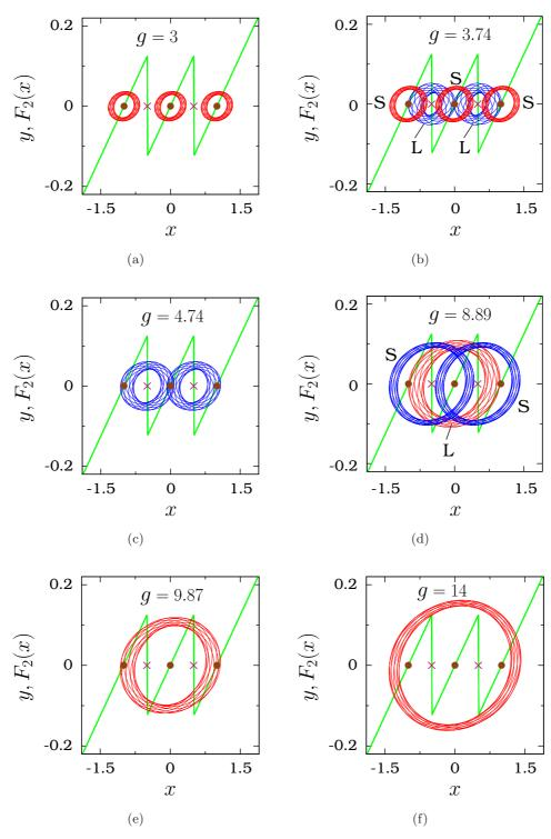
Fig. 5. Phase portraits of the coexisting orbits of the system Eq. (2) with N = 2 in the x-y plane for various fixed values of g. The solid circles and "×" mark the equilibrium points  $x^* = 0$ ,  $\pm 1$  and the breakpoints  $x^*_{bp} = \pm 0.5$  respectively.  $F_2(x)$  is also shown for illustrating the influence of the high-frequency periodic force. In the subplots (b) and (d), the value of Q for the orbits S is smaller than that of the orbits labeled as L.
