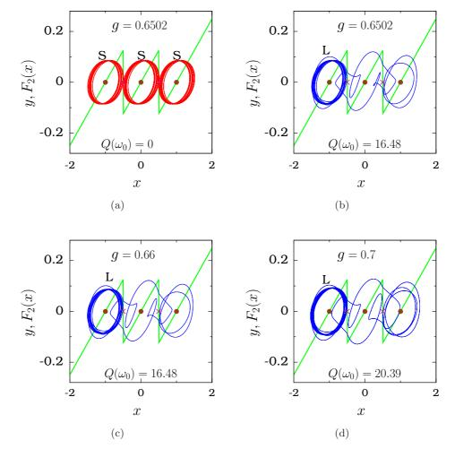
Fig. 10. Phase portraits of the orbits present at (a) and (b) the starting of the first hysteresis, (c) at the end of the first hysteresis, (d)–(f) at the starting of the second hysteresis and (g) and (h) at the end of the second hysteresis. The solid circles and the symbol " $\times$ " denote the equilibrium points and the breakpoints, respectively.  $F(x) = F_2(x)$  is also plotted.
