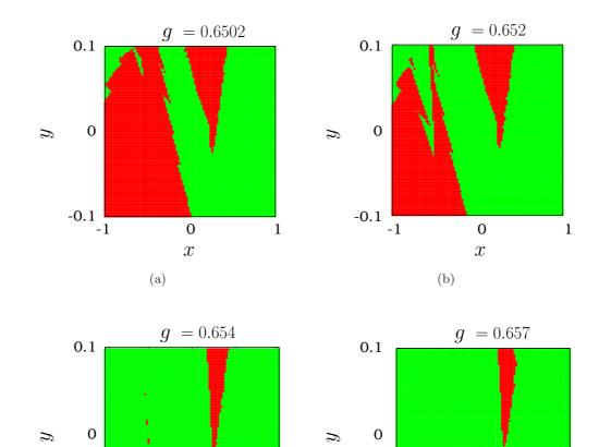
(c) (d) Fig. 11. Change in the basin of attraction of the L orbits (green colored region) and the S orbits (red colored region) for a few fixed values of g near the end of the first hysteresis in the first resonance region [shown in Fig. 9(b)]. The region  $x \in [-1, 1]$ and  $y \in [-0.1, 0.1]$  with z = 0 is divided into  $150 \times 150$  grid points.
