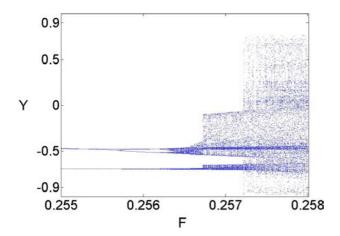
Fig. 4. Numerical bifurcation diagram  $(y=\dot{x} \text{ versus } F)$  of the Duffing oscillator in the absence of the linear spring with clearance  $(\alpha=0.15,\ k=0.2,\ h=0.3)$ . We observe periodic regions and chaotic regions depending on the value of F. The onset of chaos takes place at  $F\simeq 0.257$ .
