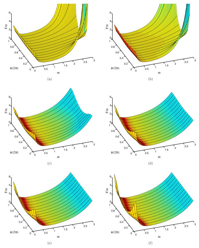
Fig. 7. The numerically estimated critical surfaces  $\eta = F/\alpha$  versus  $\omega$  that separate the regular (below the curves) and chaotic (above the curves) parameter regions for k=1 and h=1.0. The control phase  $\phi$  was chosen as  $\phi=1/4,1/3,1/2,1,2,3$  for (a), (b), ..., and (f), respectively.
