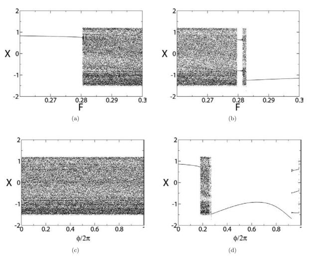
Fig. 9. Numerical bifurcation diagrams of the variable x versus F [(a) and (b)] for k=0.45 and h=1 (a) without control and (b) with control parameters:  $\varepsilon=0.2$ ,  $\phi=\pi$ . Numerical bifurcation diagrams of the variable x versus  $\phi/2\pi$  [(c) and (d)]. (c) F=0.3 without control and (d) F=0.3 with control parameters  $\varepsilon=0.2$  and  $\phi=\pi$ .
