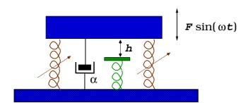
Fig. 1. Schematic plot of the two stage spring-mass model. The effective exterior springs in the figure are assumed to have the nonlinear characteristics, while the interior which introduces the nonsmoothness, has linear characteristics. h denotes the tip position of the spring free length with respect to the equilibrium point x=0.
