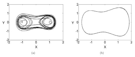
Fig. 8. Numerical plot trajectories in the phase plane  $(x, y = \dot{x})$  of the system: (a) without control and (b) with control. Parameter values are: k = 0.45, h = 1, F = 0.258 and the control parameters are  $\varepsilon = 0.1$  and  $\phi = \pi$ . We observe the clear influence of the phase to control the dynamics of our system.
