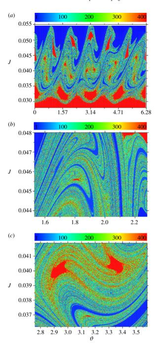
Figure 5. (a) Connection lengths for  $\epsilon = 2.14 \times 10^{-4}$ . The colour scale indicates the 'time' (measured in number of toroidal turns) it takes for a given field line to hit the tokamak wall. (b,c) Magnifications of selected rectangles in (a). (Online version in colour.)
