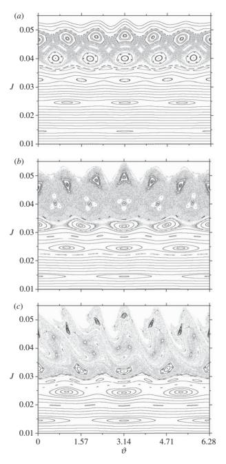
Figure 3. Phase portraits of the field line map (3.9)–(3.10) for increasing perturbation strengths: (a)  $\epsilon = 1.00 \times 10^{-5}$ ; (b)  $\epsilon = 1.20 \times 10^{-4}$ ; (c)  $\epsilon = 2.14 \times 10^{-4}$ . The upper horizontal line represents the tokamak wall.
