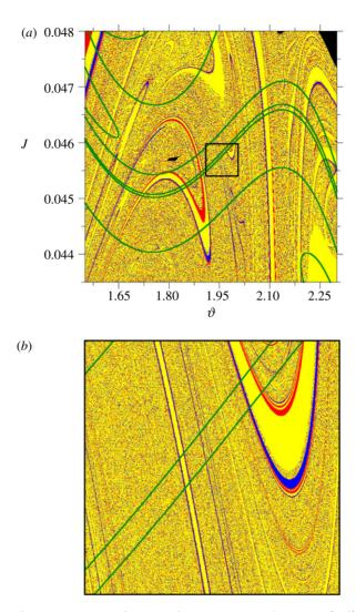
Figure 10. (a) Exit basins corresponding to the regions  $0 \le \vartheta < 2\pi/3$  (red),  $2\pi/3 \le \vartheta < 4\pi/3$  (yellow), and  $4\pi/3 \le \vartheta < 2\pi$  (blue) of the tokamak wall, for points belonging to the region shown in figure 4c. We depict in green a part of the unstable manifold stemming from the point  $P_5$  indicated in figure 7a. (b) Magnification of the box shown in (a). (Online version in colour.)
