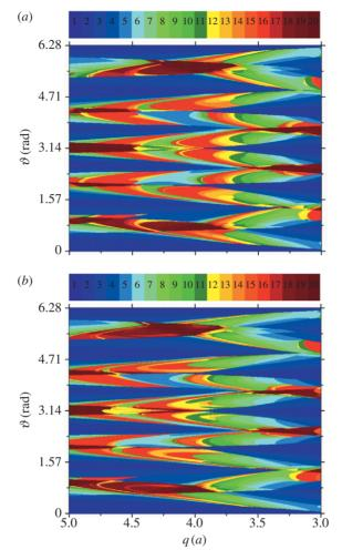
Figure 6. The colour scales indicate the connection lengths just below the tokamak wall as a function of the equilibrium safety factor at plasma edge for (a)  $\epsilon = 1.2 \times 10^{-4}$  and (b)  $\epsilon = 2.14 \times 10^{-4}$ . (Online version in colour.)
